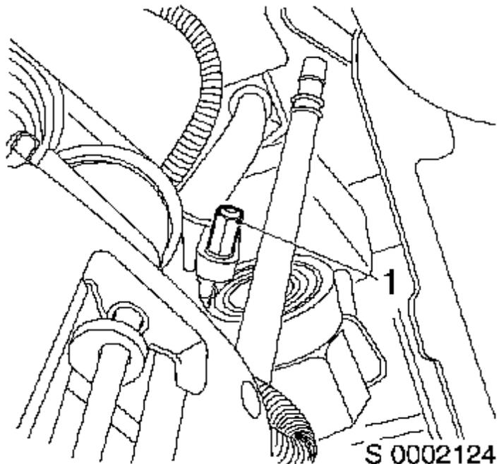
8. Release brake hose from lower wishbone
