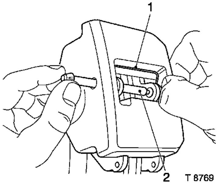
10. Tilt brake caliper upwards
